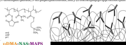
Figure 1 (a) The three major components of the polymer are DMA, NAS and MAPS in ratio 97:3:3. NAS provides the active groups, which specifically bind amine functional groups on the probe, the MAPS covalently binds to the oxide surface and DMA adsorbs to the oxide surface and provides the backbone of the polymer. (b) The polymer swells upon hydration to provide a near liquid environment for the probes. [2]
